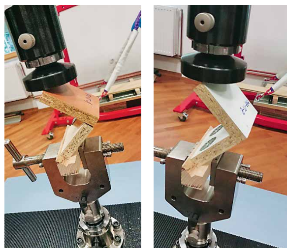
Figure 2 Testing method of bending moment for: a) RV hardware; b) Maxifix hardware Slika 2. Način ispitivanja momenta savijanja: a) okov RV; b) okov maxifix
