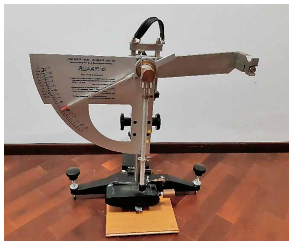
Figure 1 Pendulum test equipment for slip resistance measurement
