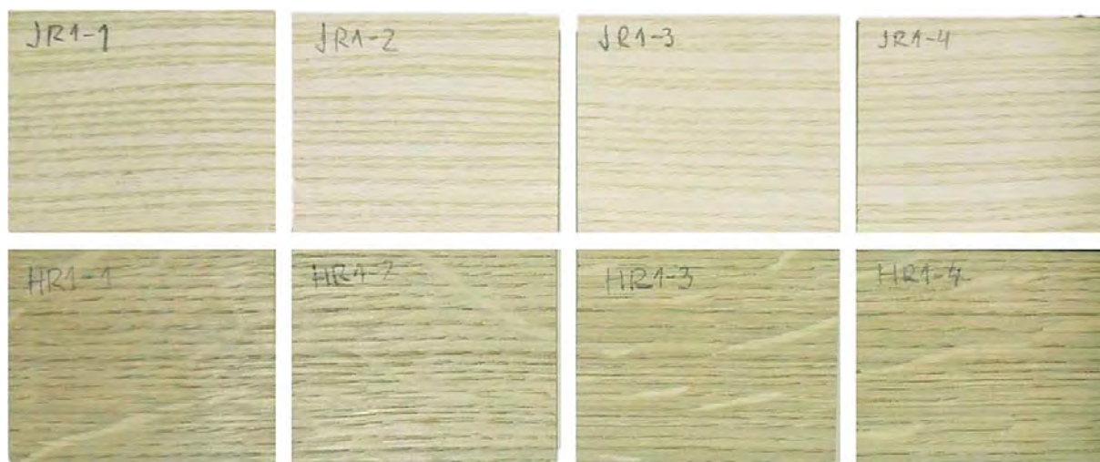
Figure 1 Parallel specimens of ash (top) and oak (bottom) for drying at temperatures of 60 °C (1-1), 70 °C (1-2), 80 °C (1-3) and 90 °C (1-4)
