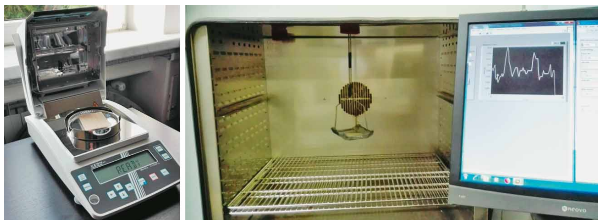
Figure 2 IR drying (left) and hot air drying experimental set-up (right)
