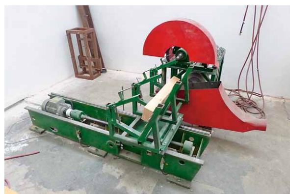
**Figure 5** Measuring equipment for cross-cutting wood
