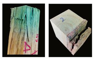
**Figure 4** Fracture modes for test specimens: Compression strength parallel to grain (left), shear strength parallel to grain (right)
