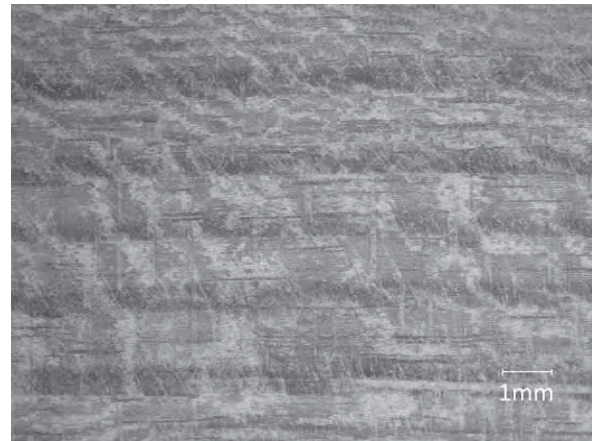
Figure 4 Scratched surface of test specimens after 1,000 revolutions in a Taber Abraser
