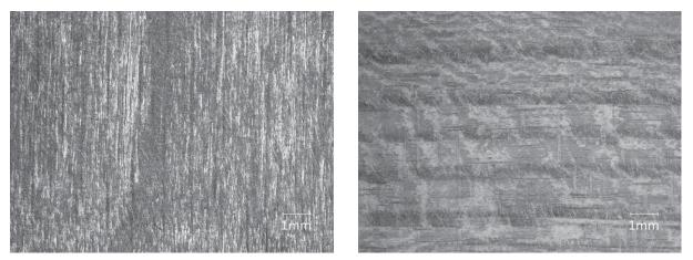
**Figure 4** Scratched surface of test specimens after 1,000 revolutions in a Taber Abraser **Slika 4.** Izgrebena površina uzoraka nakon 1000 ciklusa ispitivanja na uređaju Taber abraser
