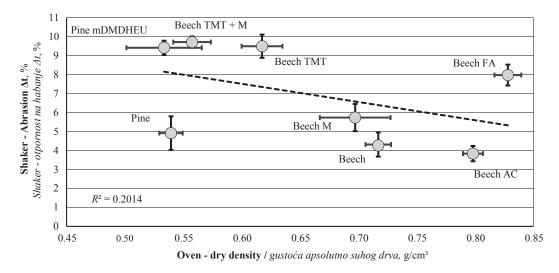
Figure 2 Relationship between oven-dry density and abrasion according to the Shaker method. Dots represent mean values per wood species. Standard deviation is indicated by error bars.
