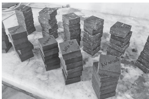
Figure 1 Water absorption and thickness swelling specimens after being immersed in distilled water for 24 hours Slika 1. Uzorci za određivanje upijanja vode i bubrenja nakon 24-satnog potapanja uzoraka u destiliranoj vodi
