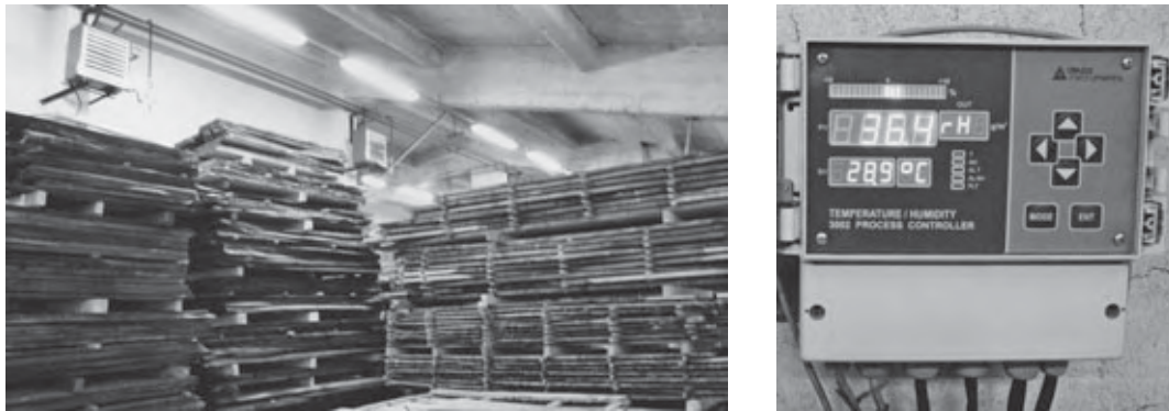
Figure 6 Automated storage house for dried wood materials (on the left) and programmable controller for automatic computation and model-based control of its conditioning process (on the right)
