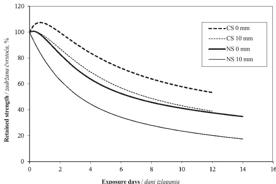
**Figure 2** Strength changes of spruce coded as Croatian spruce (CS, density 480 g/cm<sup>3</sup>) and Norway spruce (NS, density 370 g/cm<sup>3</sup>) during artificial weathering in humid conditions in QUV-2 regime
