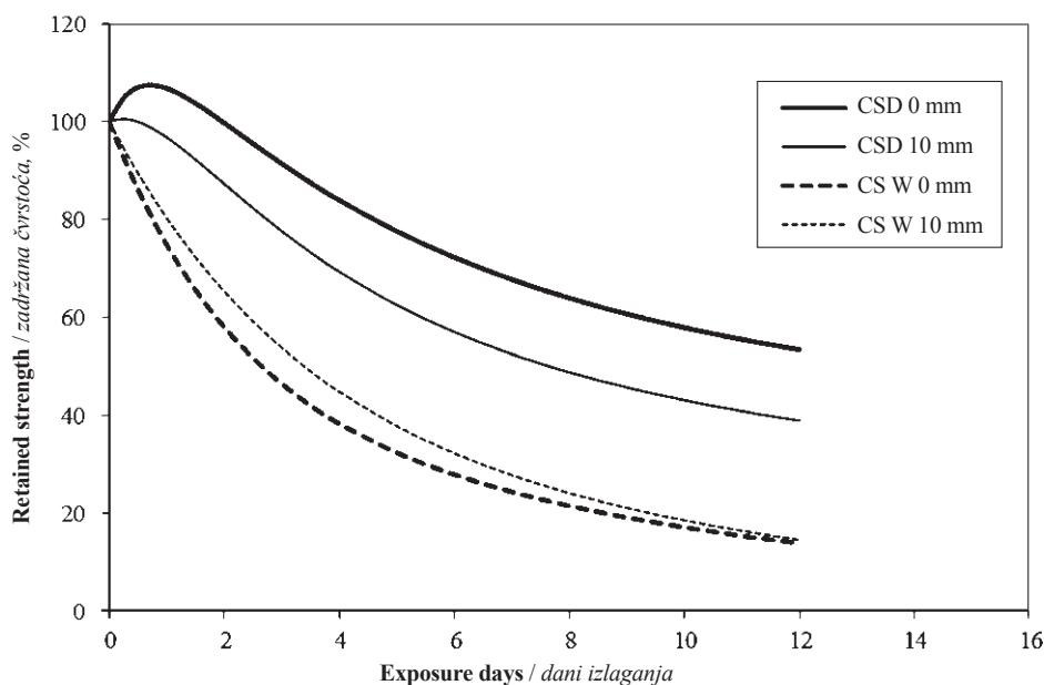
**Figure 1** The effect of wet testing of Croatian spruce (CS) on the character of tensile changes during exposure to high humidity conditions (QUV-3). Specimens were tested in dry (D) conditions (at  $20\pm1^\circ\text{C}$  and  $60\pm5\%$  RH) and wet (W), i.e. after full aspiration of water
