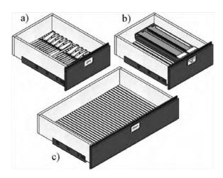
Figure 9 Middle drawers with fittings: a) a single drawer with knife holders, b) a single drawer with a foil cutter, c) a single drawer with anti-slipping mat
