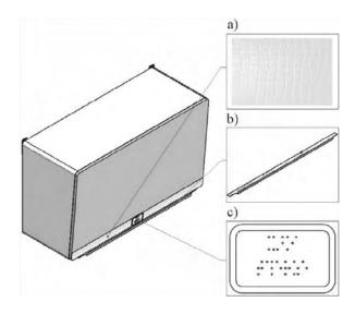
Figure 5 A hanging cabinet with improvements: a) covering, b) handle, c) the Braille space identifier Slika 5. Viseći ormarić s poboljšanjima: a) pokrov, b) prihvatnik, c) oznaka na Brailleovu pismu
