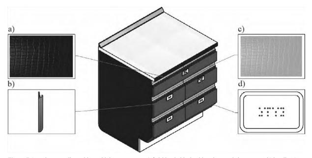
**Figure 7** A worktop standing cabinet with improvements: a) finishing in black with a characteristic structure, b) handle, c) finishing in a light colour with a characteristic structure, d) the Braille space identifier
