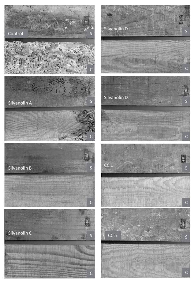
**Figure 3** Surface (*S*) and Cross-sections (*C*) of copper treated specimens exposed in the Port of Koper, Slovenia for 18 months **Slika 3**. Površina (*S*) i poprečni presjeci (*C*) uzoraka zaštićenih bakrom nakon 18 mjeseci izlaganja u luci Koper, Slovenija remained health even after 10 years of exposure in the North Sea.
