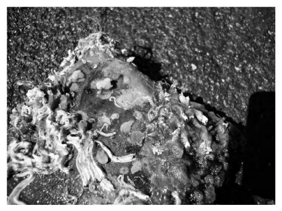
**Figure 1** Visual appearance of specimens after 10 weeks of exposure in Adriatic Sea **Slika 1**. Izgled uzoraka nakon 10 dana izlaganja u Jadranskome moru
