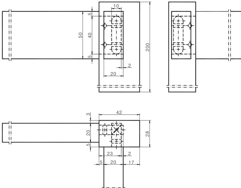
**Figure 1.** Round-head mortise diagonally shortened in tenons with lengthways hole
