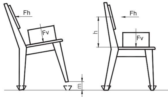
**Figure 2.** Scheme of chair testing according to standard
