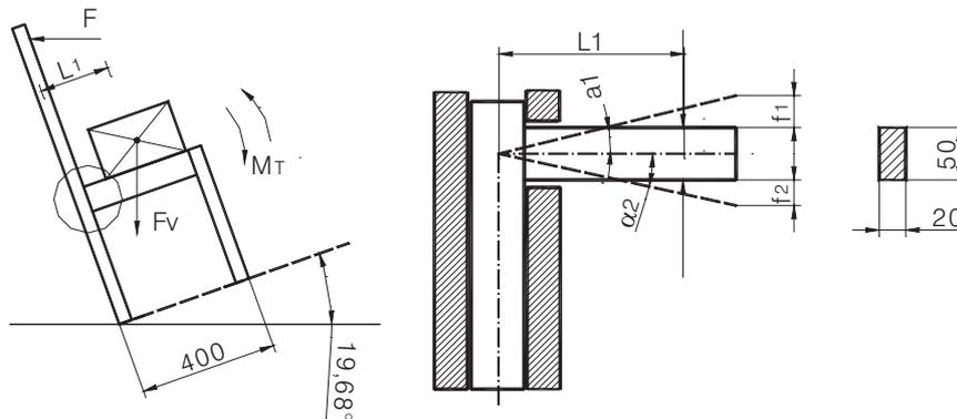
**Figure 3.** Scheme of dynamic testing samples derived from chair leg assembly
