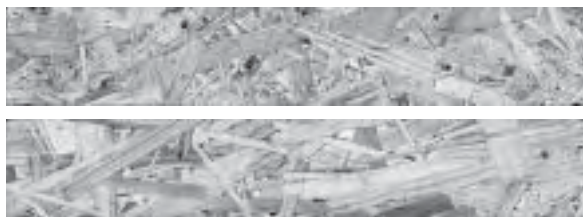
Figure 1 Top view: Lower and upper faces of OSB/3 – Superfinish, test specimens of 50 x 290 mm – parallel direction
