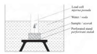
Figure 2 General arrangement of the test for measuring swelling pressure
