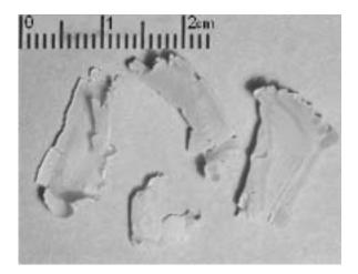
**Figure 7** The biggest fraction (above 8 mm) of chips from juvenile pine wood with angular geometry of the milling machine  $\gamma_f / \beta_f = 15^{\circ}/55^{\circ}$  and cutting parameters  $v_c = 20 \text{ m} \cdot \text{s}^{-1}$ ,  $v_f = 2.5 \text{ m} \cdot \text{min}^{-1}$
