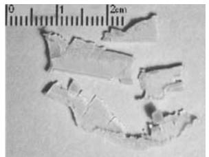
**Figure 8** The biggest fraction (above 8 mm) of chips from mature pine wood with angular geometry of the milling machine  $\gamma_f / \beta_f = 15^{\circ}/55^{\circ}$  and cutting parameters  $v_c = 20 \text{ m}\cdot\text{s}^{-1}$ ,  $v_f = 2.5 \text{ m}\cdot\text{min}^{-1}$
