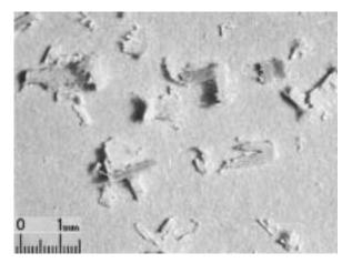
**Figure 10** The smallest fraction (under 1 mm) of chips from mature pine wood with angular geometry of the milling machine  $\gamma_f / \beta_f = 15^{\circ}/55^{\circ}$  and cutting parameters  $v_c = 20 \text{ m}\cdot\text{s}^{-1}$ ,  $v_f = 2.5 \text{ m}\cdot\text{min}^{-1}$
