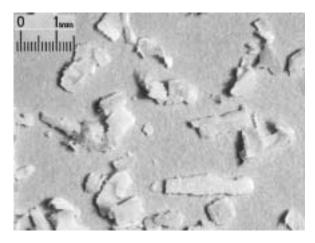
**Figure 9** The smallest fraction (under 1 mm) of chips from juvenile pine wood with angular geometry of the milling machine  $\gamma_f/\beta_f = 15^{\circ}/55^{\circ}$  and cutting parameters  $v_c = 20 \text{ m}\cdot\text{s}^{-1}$ ,  $v_f = 2.5 \text{ m}\cdot\text{min}^{-1}$
