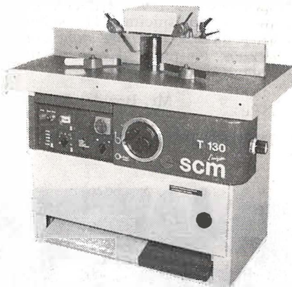
Sl. 4. Stolna glodalica SCM T 130 tvrtke SCM International
