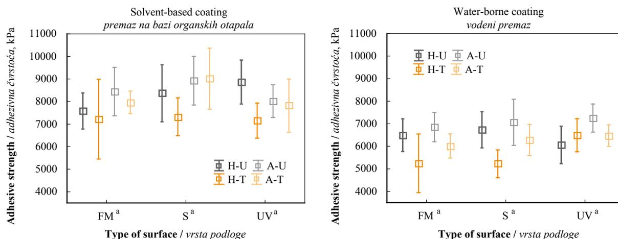
**Figure 2** Mean value and standard deviation of adhesion strength of water-borne and solvent-based coating; H-U - unmodified hornbeam, H-T - thermally modified hornbeam, A-U - unmodified ash, A-T - thermally modified ash, FM - face milled, S - sanded, UV - UV irradiated (Means within the measuring interval followed by the same letter are not significantly different at 5 % level of significance using the Kruskal-Wallis test)
