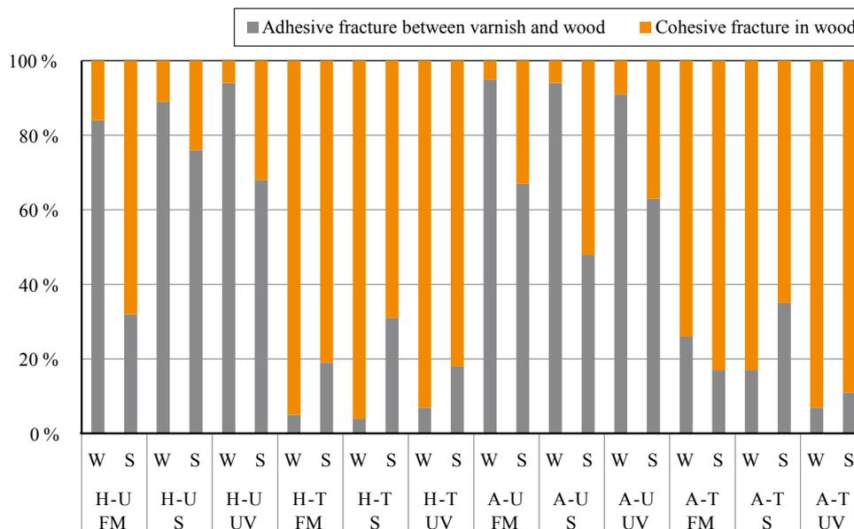
**Figure 3** Mean proportion of adhesive fracture between coating and wood and cohesive fracture in wood (W - water-borne coating, S - solvent-based coating, H-U - unmodified hornbeam, H-T - thermally modified hornbeam, A-U - unmodified ash, A-T - thermally modified ash, FM - face milled, S - sanded, UV - UV irradiated)
