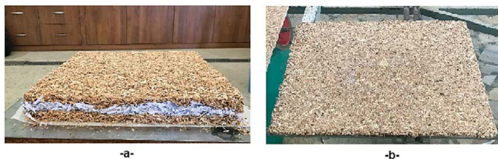
Figure 3 Hot-pressed board: (a) pre-hot pressing, (b) post hot pressing
