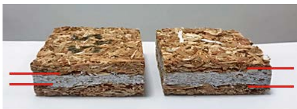
Figure 9 Separation between layers after water absorption-thickness swelling test
