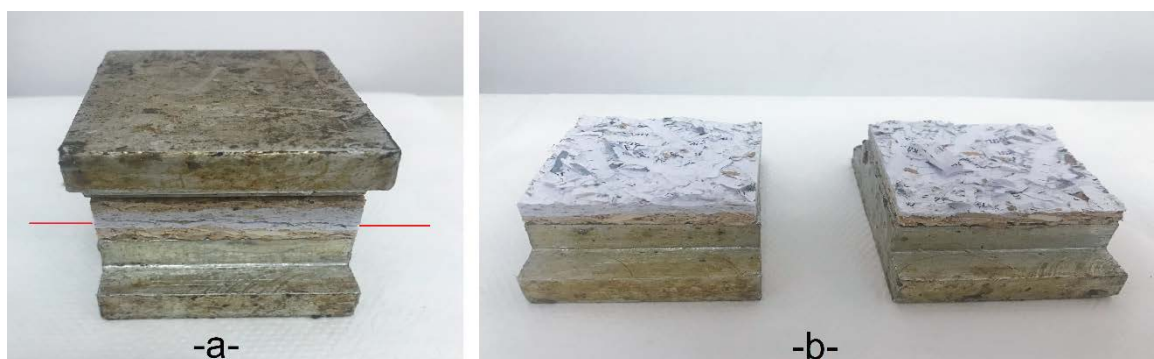
Figure 7 Results of internal bond strength test: (a) middle layer, (b) failure type after rupture
