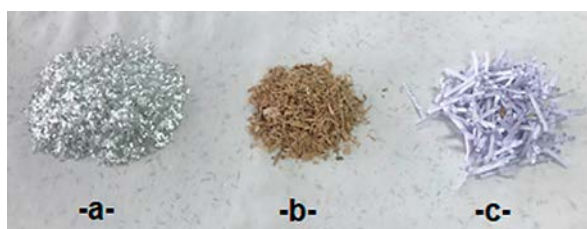
Figure 1 Materials used in the study: (a) chopped glass fiber, (b) wood chips, (c) office waste paper
