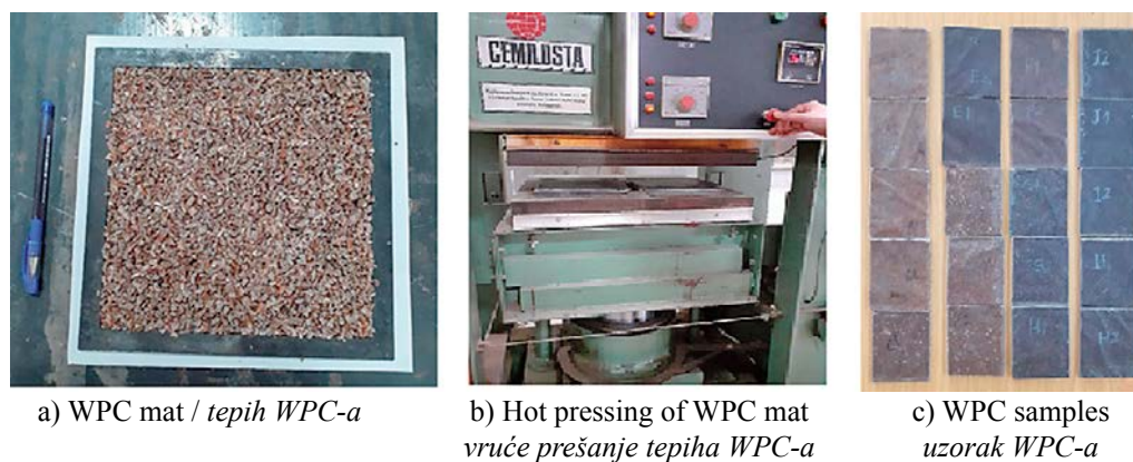
Figure 2 Hot-press molding of WPC granules and resulting WPC specimens Slika 2. Vruće prešanje WPC peleta i dobiveni WPC uzorci
