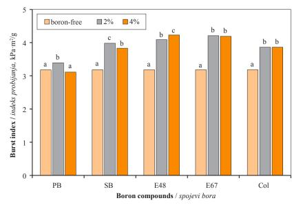
**Figure 4** Effects of boron compounds on burst index of pulps **Slika 4.** Utjecaj spojeva bora na indeks probijanja celuloze
