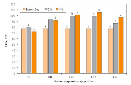
**Figure 3** Effects of boron compounds on TEA of pulps **Slika 3.** Utjecaj spojeva bora na TEA celuloze
