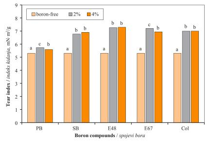
**Figure 5** Effects of boron compounds on tear index of pulps **Slika 5.** Utjecaj spojeva bora na indeks kidanja celuloze
