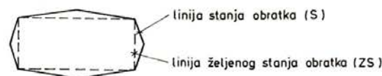
Slika 5. Obradak oblikovan s po dva zuba na više strojeva Fig. 5 — Workpiece formed with two teeth on each of several machines
