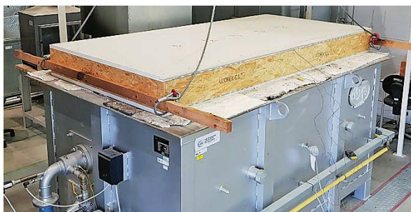
Figure 1 Experimental fire furnace with test specimen TS1 (photo: authors)
