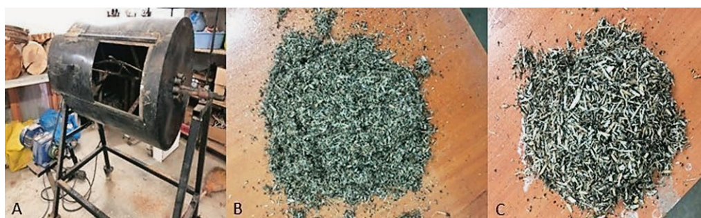
Figure 1 A) Gluing machine, B) Surface layer blend, C) Core layer blend
