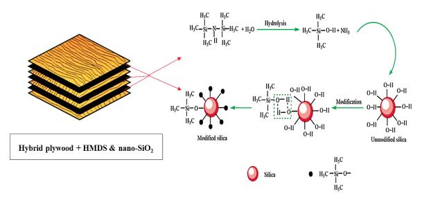
Figure 1 Schematic diagram showing influence of nano-SiO2 modified by HMDS on bonding of rubber between wood layers (Song *et al.*, 2014)
