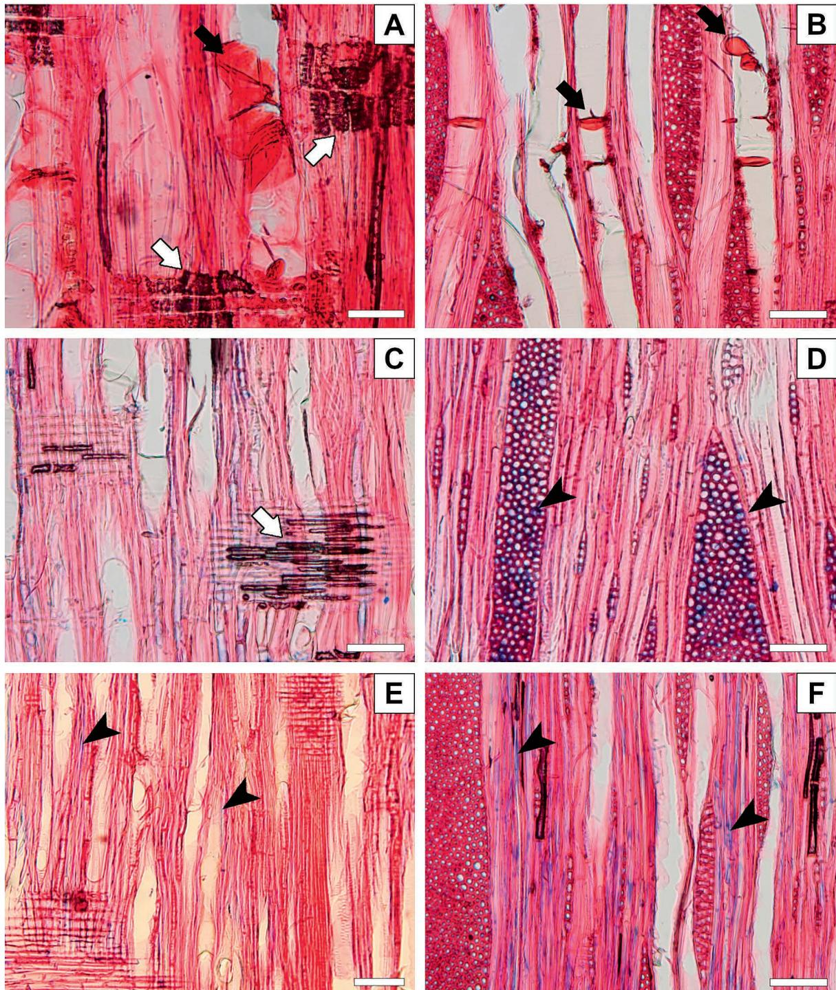
**Figure 6** FHW (A and B), RW (C and D) and SW (E and F) microsections stained with Astra Blue and Safranin stain combination. A, C and E are radial microsections and B, D and F are tangential microsections. Scales are denoted with a white stripe in the lower right corners of the figures – 50  $\mu\text{m}$  in 5A and 100  $\mu\text{m}$  in the other figures.
