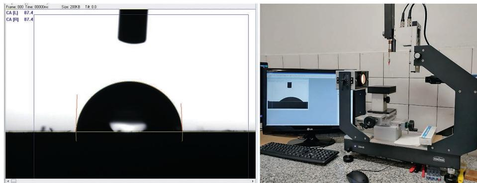
**Figure 1** Contact angle measurement by the circle method on the left side of the figure; Krüss DSA30 Standard drop shape analyzer on the right side of the figure**Slika 1.** Mjerenje kontaktnog kuta kapi (lijeva slika); Krüss DSA30 standardni analizator oblika kapi (desna slika)
