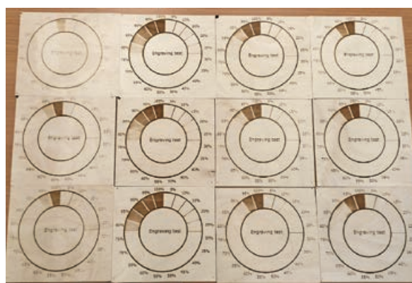
Figure 6 Results of an engraving test and changes in discoloration of birch plywood at \Delta F = - 8 mm
