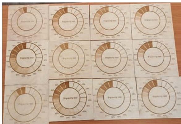
Figure 4 Results of an engraving test and changes in discoloration of birch plywood at \Delta F = - 4 mm
