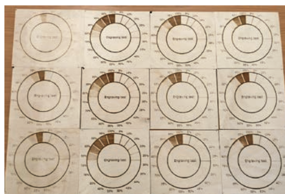
Figure 5 Results of an engraving test and changes in discoloration of birch plywood at \Delta F = - 6 mm
