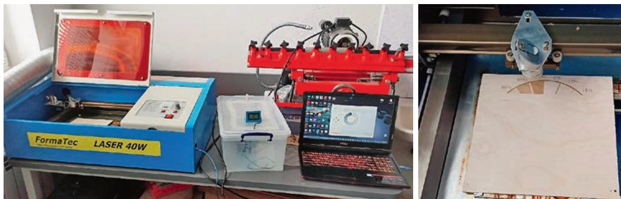
Figure 2 CO 2 laser machine for engraving and cutting Slika 2. CO 2 laser za graviranje i rezanje
