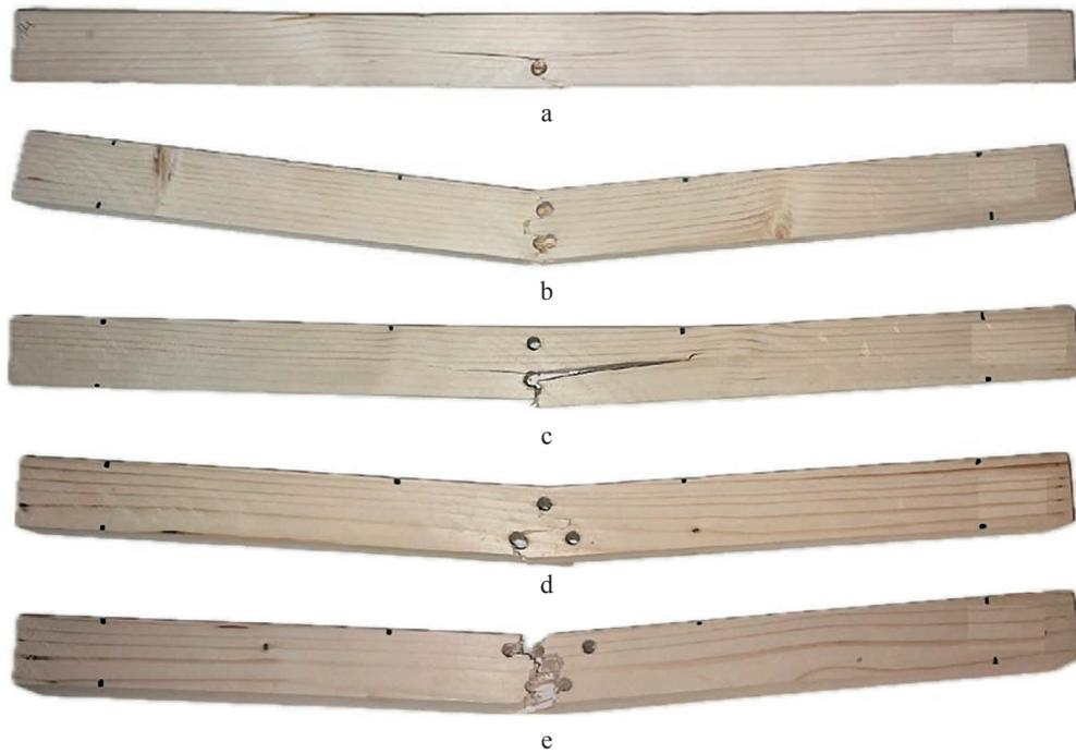
**Figure 4** Typical specimen fracture cases
