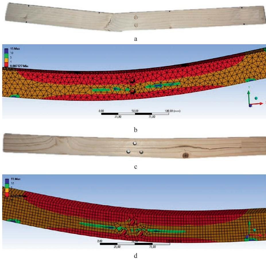
**Figure 5** Examples of stress distribution simulated by design program for specimen failure (a, b – one from group III, c, d – one from group V)
