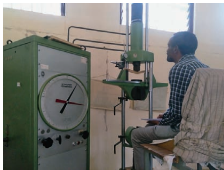
Figure 2 Universal testing machine (UTM) for static bending test
