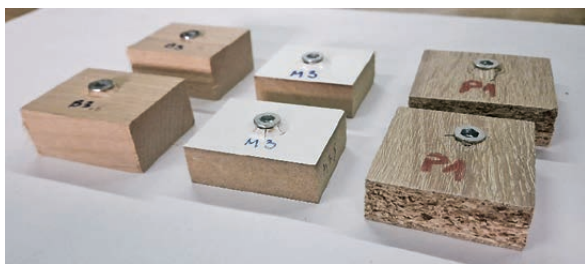
Figure 11 Failures caused by withdrawal force of double-threaded nuts mounted into beech wood, MDF, and particleboard
