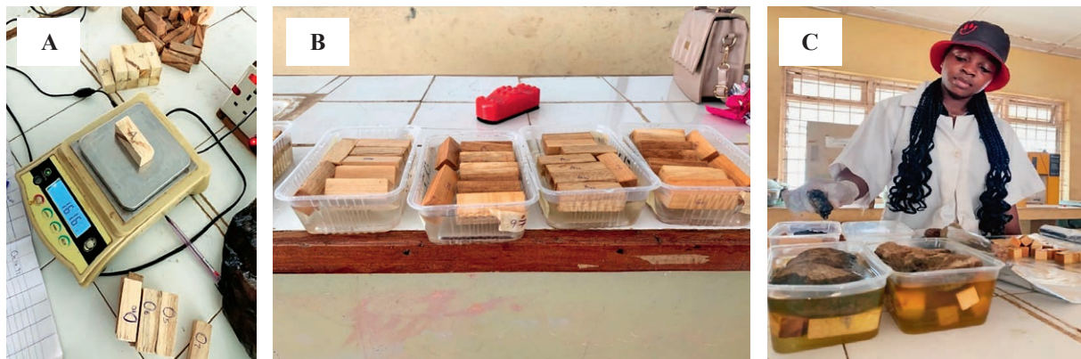
Figure 3 Experimental procedures for physical properties test: A) weighing of wood samples B) extracted samples prepared for test C) soaking of samples in water
