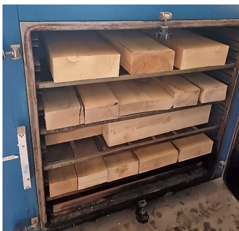
Figure 1 Stacking in heat treatment furnace
