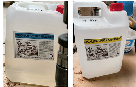
Figure 2 Scalica epoxy adhesive system resin (A) and hardener (B)
