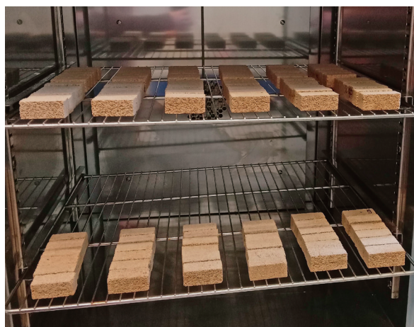
Figure 2 Composite material specimens during the drying process in an oven at 103 ^\circ\text{C}
