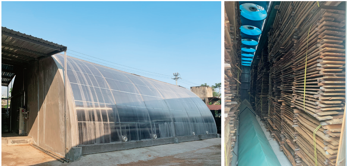
Figure 1 Schematic diagram of the experimental solar–steam hybrid wood drying system: a) Exterior view of the kiln; b) Interior view of the kiln during drying
